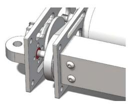
**Step 21:** Install Spacers (am-2650) on either side of the assembly, between the Cap Plate and Base Plate. Install 4 - 1/4-20 SHCS (am-1012) and Nylock Nuts (am-1015), through corner holes on Cap Plate, Base Plate, and Spacers, using 3/16" hex wrench and 7/16" wrench.
