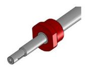
**Step 4:** Apply thread lock adhesive on the Brass Nut and Ram Cap outer threads. Apply a small amount of grease to the lead screw. Hold the flats of the Ram Cap in a vice with a rag to protect marring on the Ram Cap. Screw the Ram Cap onto the Ram Tube while also threading it onto the Brass Nut. Use a ¾ wrench to tighten the Rap Cap.
