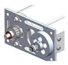
**Step 17:** Install Pivot Block (am-3249) on outside of Cap Plate, using 2 - #10-32 SHCS (am-1120) and 5/32" hex wrench. The outside of the Cap Plate is identified by the counter bore on the center hole in the plate (that is where the potentiometer is installed).
