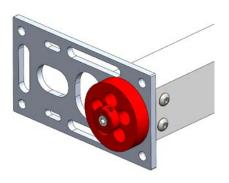
**Step 8:** Slide the Ram End into the Square Tube so the tapped holes on the Ram End Bearing align with holes on the Square Tube. Use red thread lock adhesive on 8 - #10-32 BHCS (am-1028) into the Square Tube onto both sides of the Bearing Block and the Ram End Bearing.
