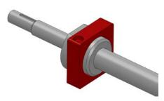
**Step 5:** Press the one of the 3/8" ID bearings (am-0209) into a pocket of the Bearing Block. Insert the 1/4" long, 3/8" id aluminum spacer (am-3260) into the middle of the Bearing Block. Press the other 3/8" ID ball bearings into the Bearing Block pocket. Keep the spacer hole and the bearing holes aligned.
