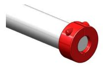
**Step 3:** Insert the Back Block (am-3255) onto the Brass Nut, leading with the smaller interior shoulder fitting on the Brass Nut threads. Press the Back Block all the way to the flange of the nut. This may be a tight fit, and can be screwed or tapped into position with a small hammer.
