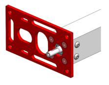
Step 11: Slide the 30 tooth HTD pulley (am-3265) onto exposed end of lead screw, aligning keyway onto machine key, until pulley touches the aluminum spacer. Mount the 5/16" collar clamp (am-2383) onto exposed end of lead screw.
