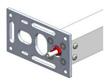
Step 12: Slide R3 Bearing (am-0031) and 14T Gear (am-3268) onto Shoulder Screw (am-1388), with Bearing nearest the Shoulder Screw head. Using red thread lock adhesive, screw Shoulder Screw into the end of the DART Lead Screw.
