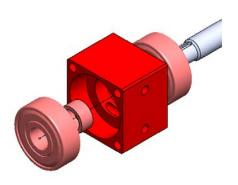
**Step 2:** Install Brass Nut (am-3262) onto Lead Screw (am-3257) with flange closest to the narrow end of the screw. Position nut so that the flange face is even with end of threads of the lead screw.
