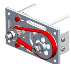
Step 18: Install potentiometer (am-2619) onto Cap Plate (am-3250), using 1/2" wrench, with counter bored portion of plate facing blue potentiometer body. Position the lock washer included with the potentiometer between the nut and the Cap Plate.
