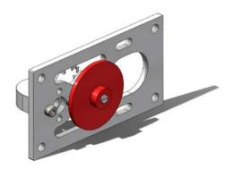
**Step 20:** Install Cap Plate onto DART assembly so that the R3 bearing on the end of the lead screw fits into the bearing hole on the Cap Plate. The plastic potentiometer gear will need to move slightly in order to nest the R3 bearing into the hole. This plastic gear needs to mesh with the 14 tooth gear on the lead screw shaft, but not rub against the heads of the adjacent #10-32 screws.
