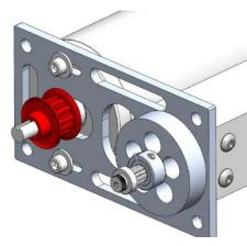
Step 16: Install the 48 tooth HTD timing belt (am-3274) onto both pulleys. Pull the CIM Motor away from the Square Tube so that the belt is tight on the pulleys. Make sure the belt teeth engage both pulleys. Tighten the 2 - #10 SHCS to fasten the CIM Motor in place.
